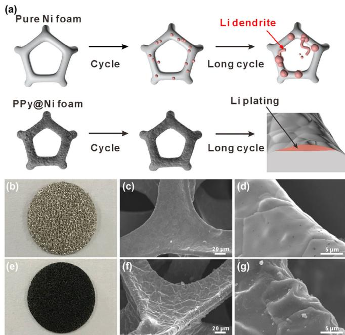
**Figure 1** (a) The schematic illustration of different Li deposition process. Optical photographs of (b) pristine Ni foam and (e) PPy@Ni foam. SEM images of (c) and (d) pristine Ni foam and (f) and (g) PPy@Ni foam.
