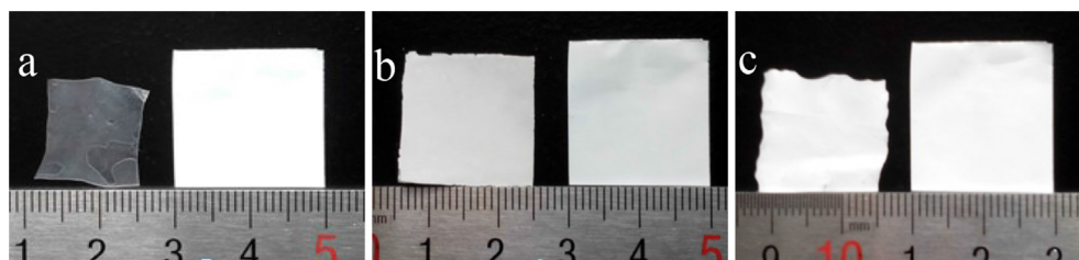
Fig. 3. Dimensions of separators before and after subjected to heat treatment at 150 °C for 30 min (a) pristine PE separator; (b) ST coating separator; (c) SP coating separator.
