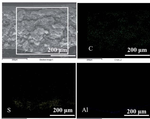
Fig. 2 Elemental mapping of the cross-section of the Al-S-VGCF electrode (sulfur areal loading of  $\sim 5 \text{ mg cm}^{-2}$ ).
