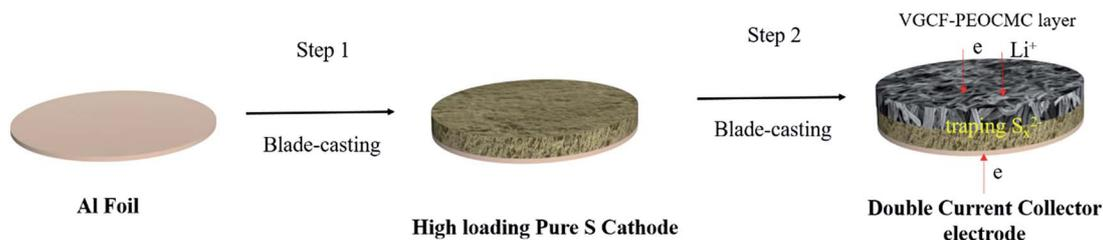
Scheme 1 Schematic of the fabrication of the Al-S-VGCF double current collector electrode.
