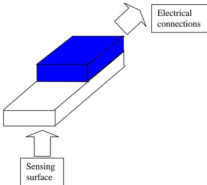
4. electrical connections from the heat spreader should all be routed to exit from one end of the heat spreader and should be routed AROUND heating elements rather than be allowed to lie over the top of them. If allowed to lie over the heaters, direct heating of the temperature sensors will become possible and the cables could prevent good contact between the heaters and the enclosed battery.
