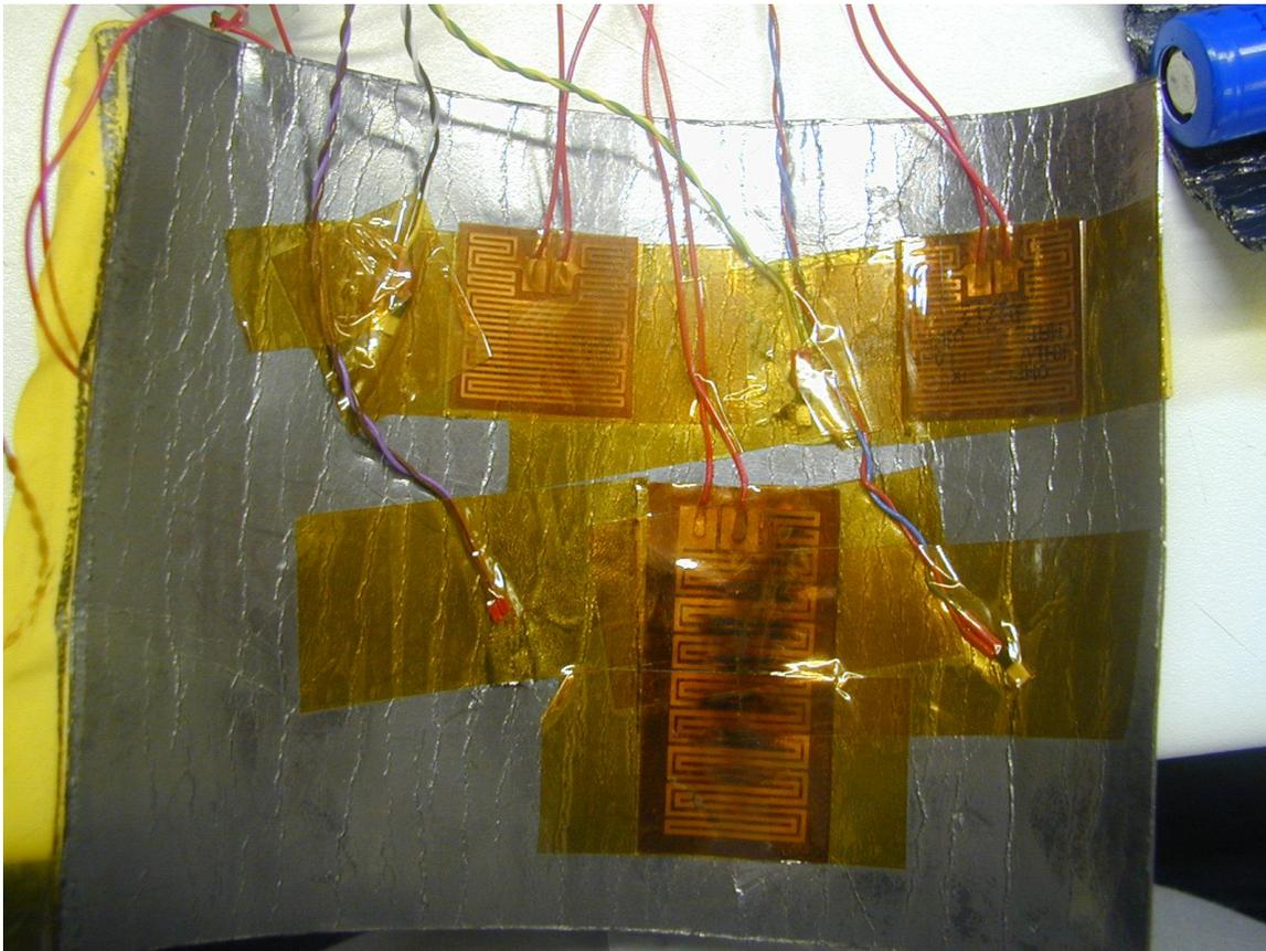
When supplied thermal control assemblies will have heaters and temperature probes already connected to an appropriately sized and shaped template of heat-spreader material
