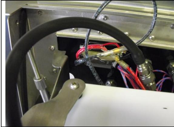
4) the connector from the battery assembly can then be connected to the mating connector mounted in the top left hand corner of the battery enclosure back plate.
