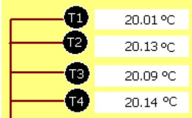
Shows the various measurements of battery temperature – returned from a number of sensors distributed around the battery. Four sensors are typically available (T1-T4) and these are averaged to give the “Battery temperature” which is used as feedback in all temperature control.
