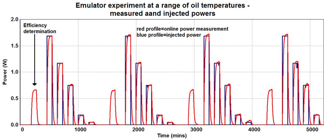
It is clear that the agreement in this case is very good – it is also apparent that the power measurement is unaffected by the changes in oil temperature. The relationship between the injected and measured power for the four values of oil temperature are summarised in the figure below – the multiple datasets are coincident.
