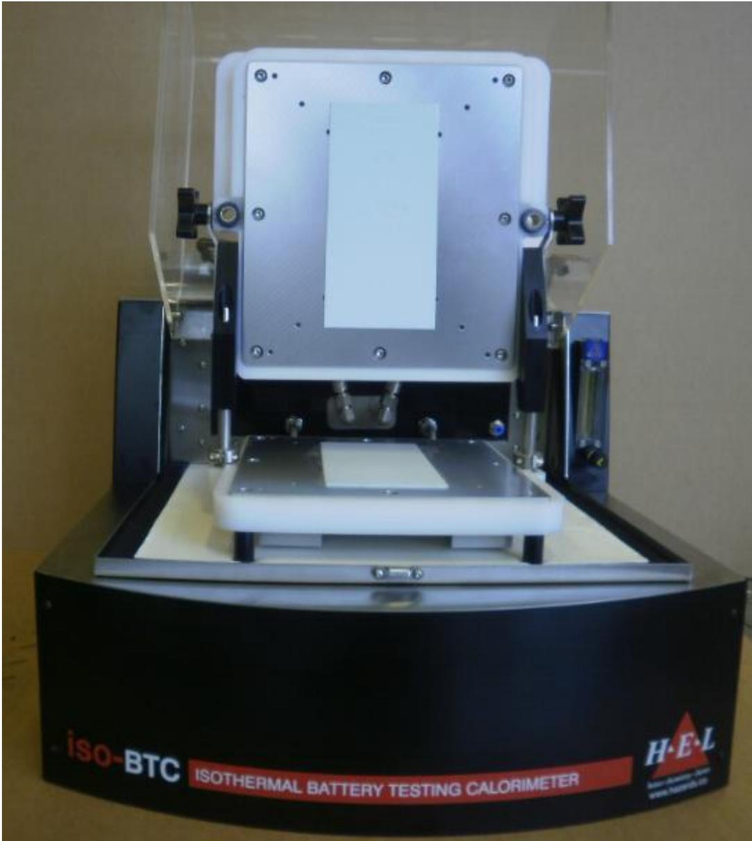
The electronic systems of the iso-BTC are responsible for measuring the battery temperature(s), controlling the heaters which are used to control this battery temperature, monitoring the voltages of individual cells in the battery and measuring battery voltage and current during charge and discharge.
