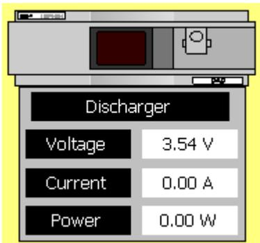
While labelled as presenting battery discharge data the voltage field (read by sense lines attached directly to the battery terminals) gives a reliable indication of the battery terminal voltage at all times. On double clicking in any of the dischargers numeric display panels a dialog box is displayed which allows the discharge to be activated and its discharge level set.
