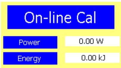
These fields show the real-time calorimetry data “Power release” and “Energy release” determined by the WinISO on-line calorimetry system. NOTE: these values are estimates while the calculation is actually running in that they do not incorporate baseline interpolation i.e. there will be no adjustment for baseline shift during the “heat release”. Such adjustments are applied as the data is written at the end of the experiment.
