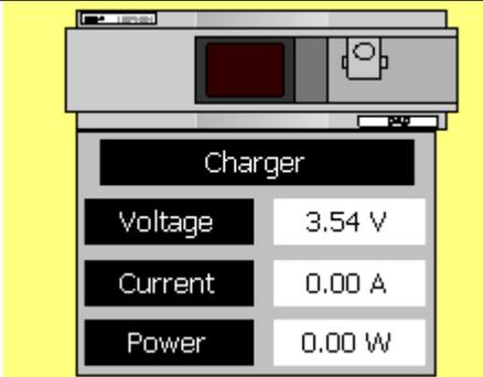
These data are typically read directly from the battery charging unit (either a separate PSU or a component of the incorporated battery cycling unit). Exact behaviour will depend on the cyclers being used but typically the voltage and current fields will only display the current battery condition when the charger is active – at other times typically showing the last used charging parameters.
