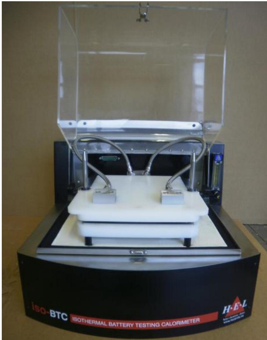
To install or remove a battery from the Iso-BTC the top plate can be lifted and supported on the *bottom plate retaining studs* (as shown in the photograph below).
