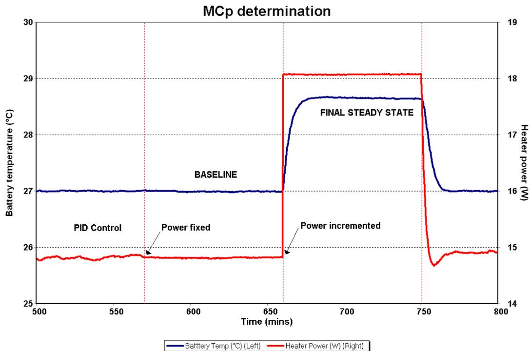
From the data above, considering **only the mass of aluminium in the sample**, the following results are obtained.
