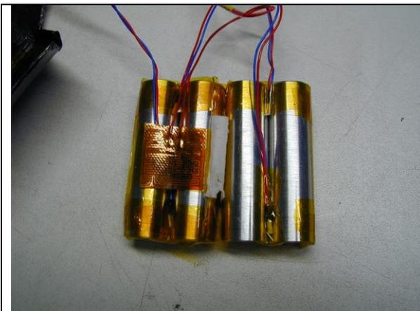
In the image to the left, four 18650 “batteries” will be used to assemble a prismatic stack. The batteries are grouped in pairs – the calibration heater is visible, fixed to the left hand pair of batteries. The four PT100 sensors with their connecting wires are visible, with two fixed to each pair of batteries
