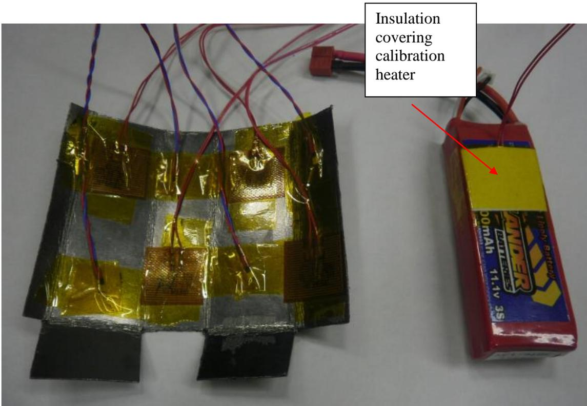
When wrapped around the battery and fixed using a suitable temperature resistant but thermally conductive tape<sup>5</sup> the battery and its spreader constitute a simple assembly which can be plugged into the BTC control system via a single connector. This assembly for the prismatic battery shown above can be seen in the image below.
