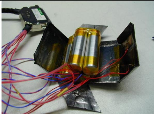
The heat spreader can be folded around the battery stack – a hole in one end allows the heater and temperature probe connections to be fed out for connection to the multi-way connector at the back of the Iso-BTC. This process is illustrated in the figure to the left.
