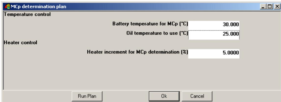
The required battery temperature should be entered in the relevant field. An oil temperature approximately 5°C lower than the requested battery temperature should be entered. The heater increment can be left at 5%, although for very large battery stacks where this gives too low a temperature rise to measure accurately, this increment can be increased.
