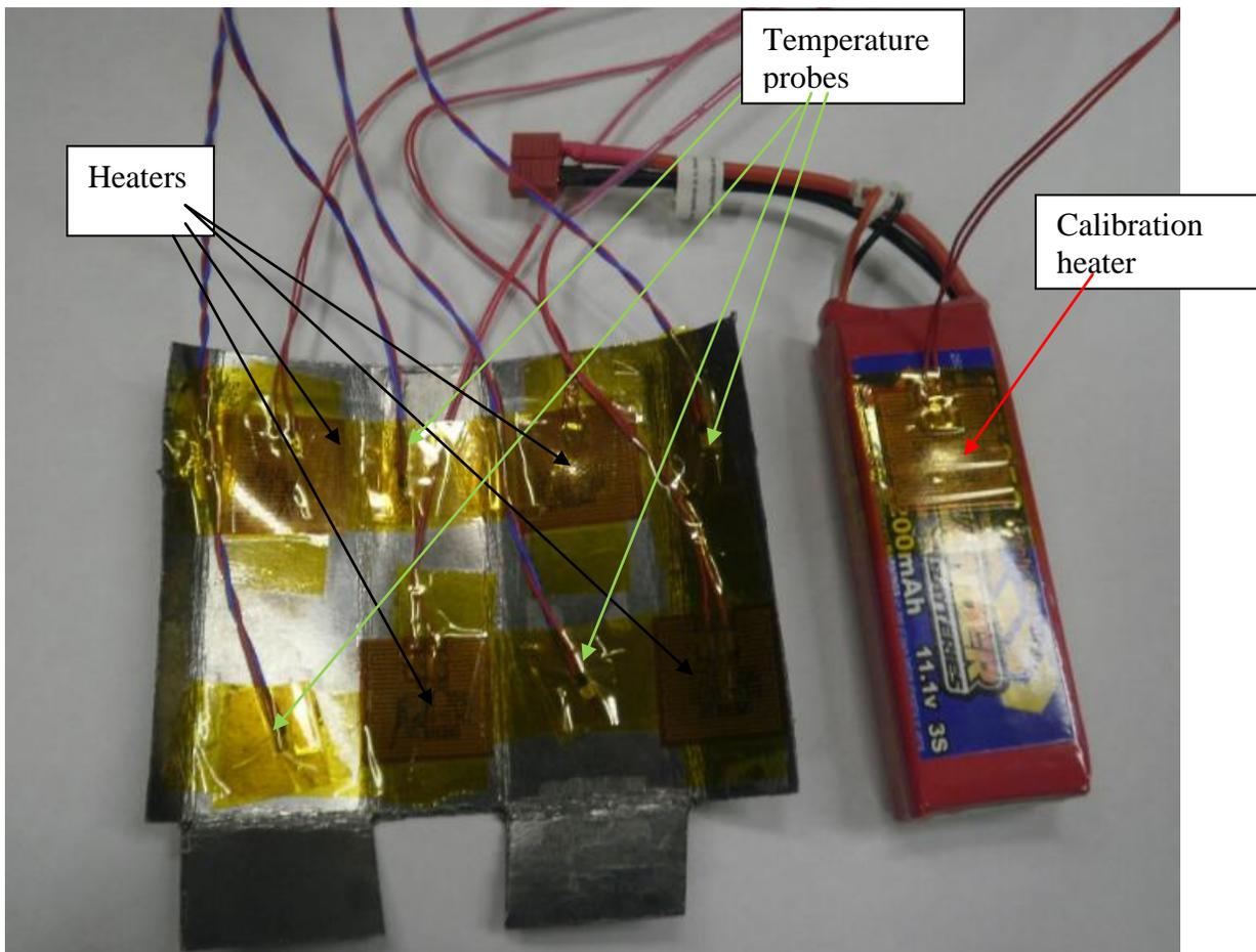
The calibration heater pictured in the image above (and the following image) is used for the online evaluation of efficiency. This, and alternate strategies for efficiency determination, are described later in this document.
