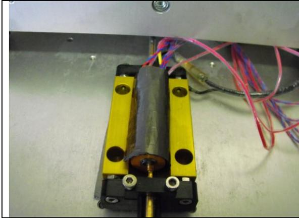
The battery/ thermal control assembly positioned in its adapter in the Iso-BTC.
