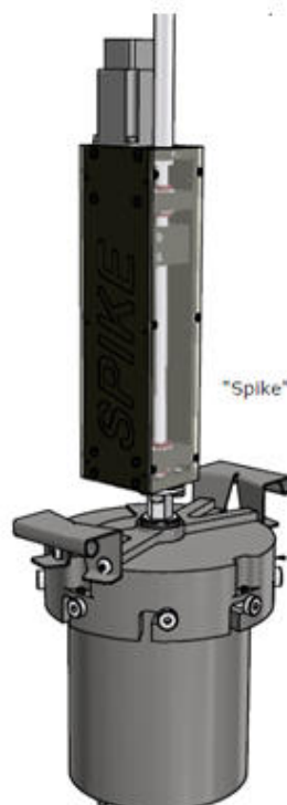
BTC130 with Nail Penetration Option
