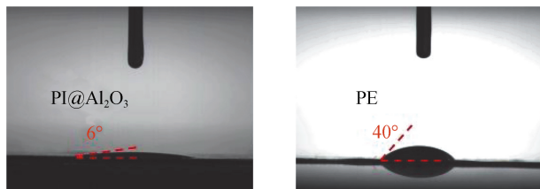
图 2 前驱体溶液在 PI@Al 2 O 3 隔膜和 PE 隔膜表面上的接触角 Fig. 2 Contact angle of precursor solution on the surface of PI@Al 2 O 3 separator and PE separator
